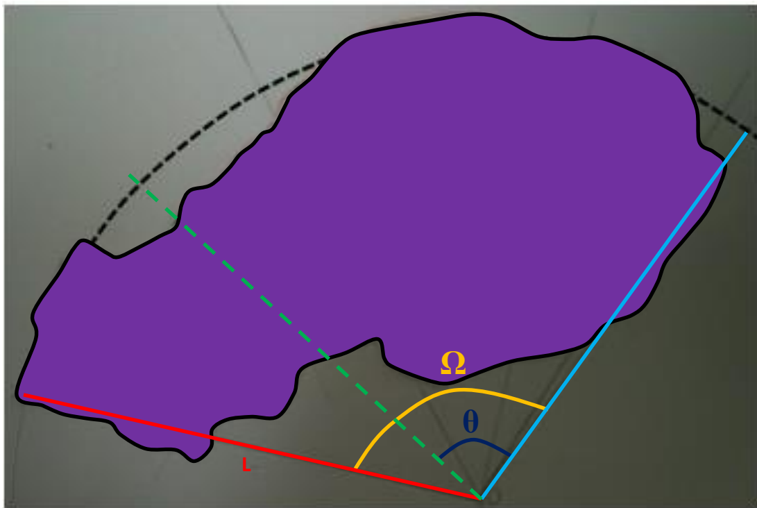
Figure 70: LV paper band trace. Red line: Starting line, Blue line: Ending line of the idealized band. \Omega is the total band angle and \theta is the angle subtended by the band for one conic rotation
