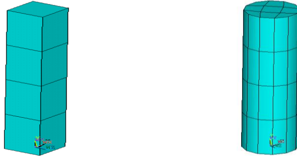
Figure 59: Number of elements generated using mapped meshing in case of a square cross-section is much less than in case of circular cross-section
