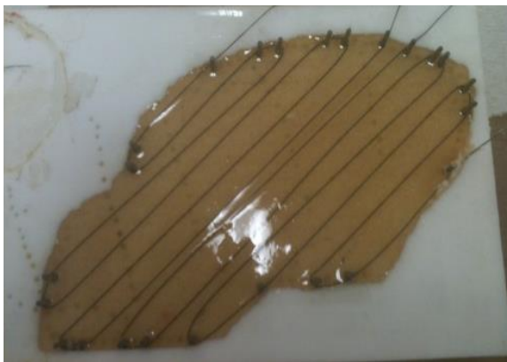
Figure 23 (A): The idealized PU/SMA flexible-matrix composite band [9] Figure 23 (B): The final conical LV-like structure [9]
